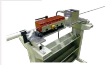
T-DRILL cutting machines can be equipped with tube pre-straightening equipment as well as NDT (Non Destructive Testing) or color detecting equipment that remove bad sections from the coiled tubing automatically during the cutting process
