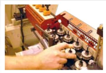
Tube straightener consists of vertical and horizontal rolls (7+7 or 9+9) and it can be equipped with digital readout for easy setting. Straightening rolls can be also changed without tools with an optional quick changing system.
