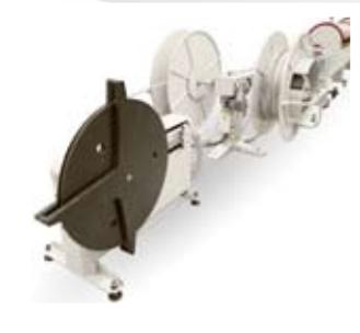
Tubing can be fed from different types of single or double coil holders with different types of coils (cardboard, bulk and capillary) for different applications
